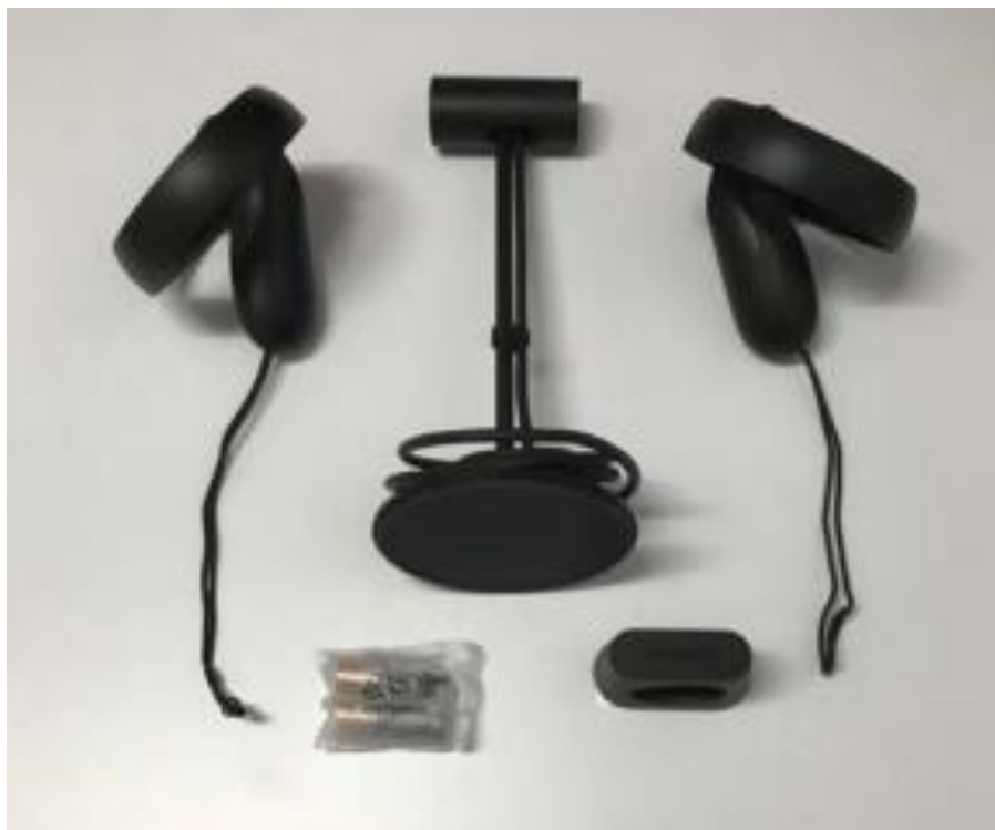
Visual 4. Other equipment of the VR set (sensors-Controllers-battery-adapter)
